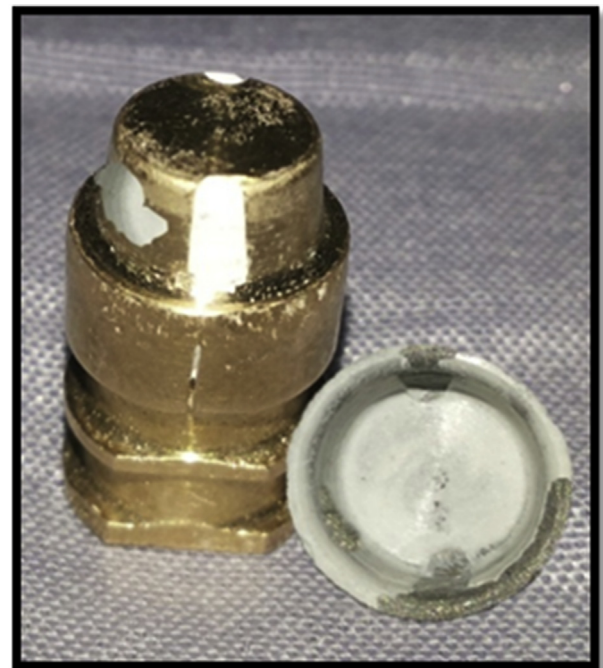
Fig. 6. The retained cement inside the frustum (Gr. F).
