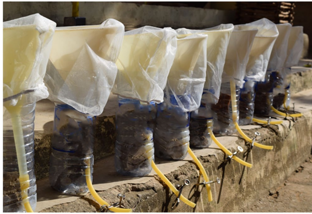
Figure 2. Modified Baermann funnels for sedimentation and recovery of suspect D. medinensis larvae from muscle tissues of fish and amphibians in Chad, Africa (photo courtesy of C.A. Cleveland).
