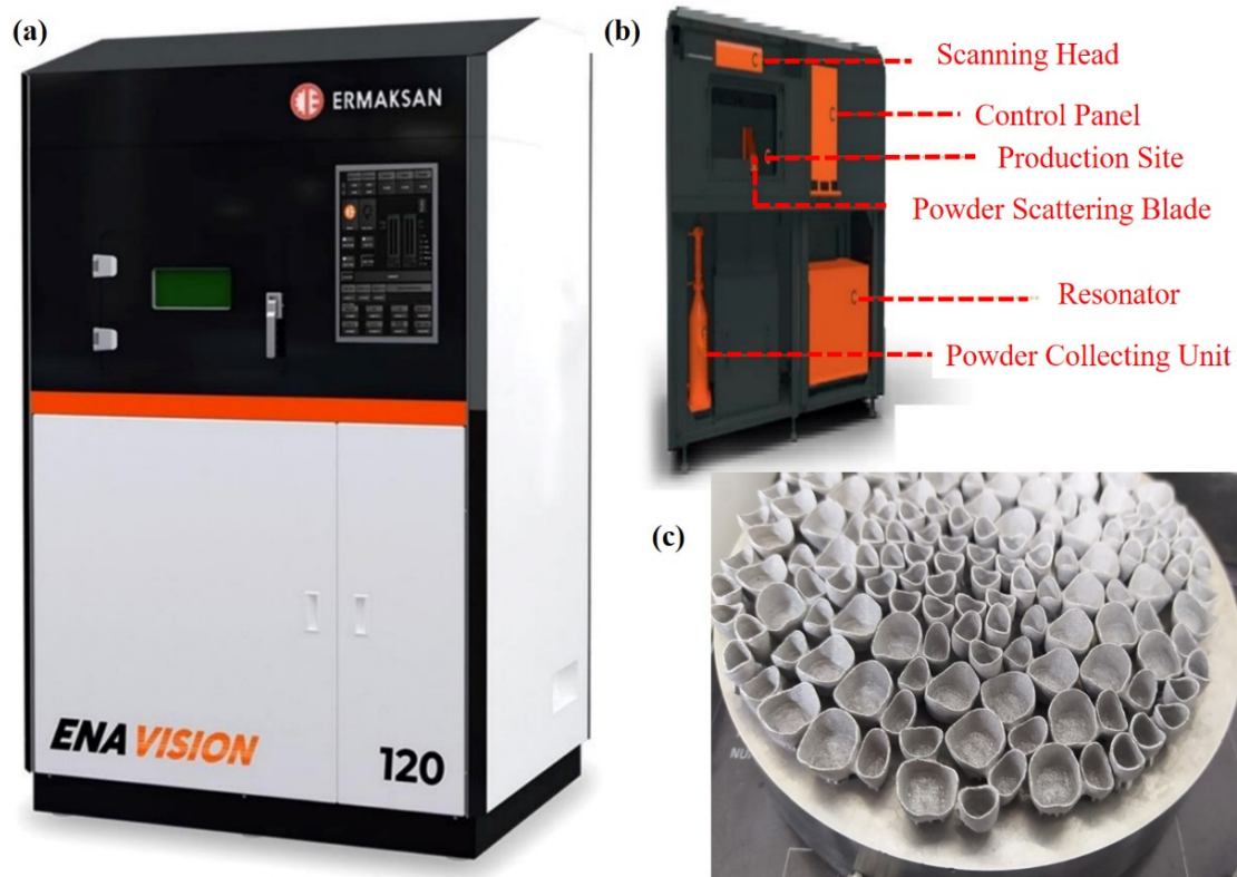
Figure 3. (a) ENAVISION 120 machine, (b) nomenclature of the machine, and (c) Co–Cr specimen printed by LPBF.
