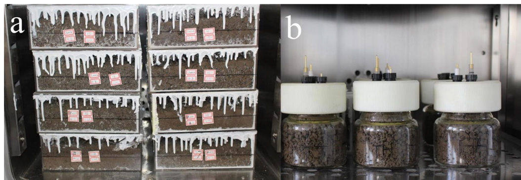
Figure 1. (a) The labeled soil reactors filled with soil samples burying coupons; (b) the electrochemical cell filled with soil samples.
