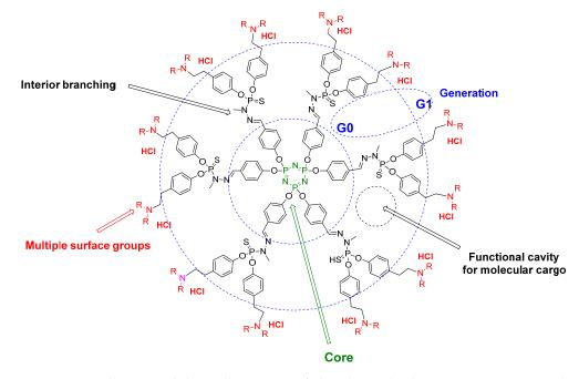
Figure 1. Two-dimensional chemical structures of phosphorus dendrimers: generations 0 and 1.
