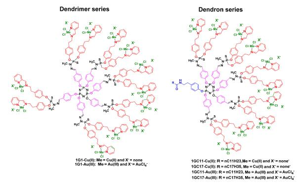
Figure 5. Schematic 2D chemical structures of dendrons 1GC<sub>11</sub>-Cu(II), 1GC<sub>17</sub>-Cu(II), 1GC<sub>11</sub>-Au(III) and 1GC<sub>17</sub>-Au(III), dendrimers 1G1-Cu(II) and 1G1-Au(III).
