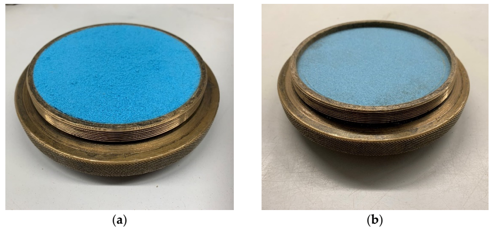
Figure 9. Sample of kinetic sand in the container of oedometer apparatus. (a) Original sample before testing; (b) Boiled sample after testing.
