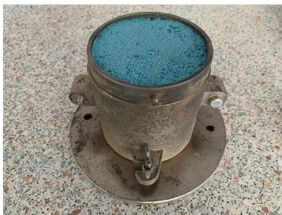
Figure 8. Steel cylindrical container with kinetic sand sample before compaction.
