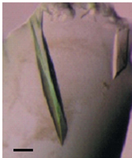
Figure 1 Tm-1(431) crystals. The typical crystal dimensions are approximately 0.6 × 0.3 × 0.07 mm. The scale bar indicates 0.1 mm.
