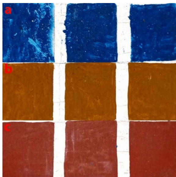
Fig. 2. The prepared samples before put the rusty nails touching the color surface.
