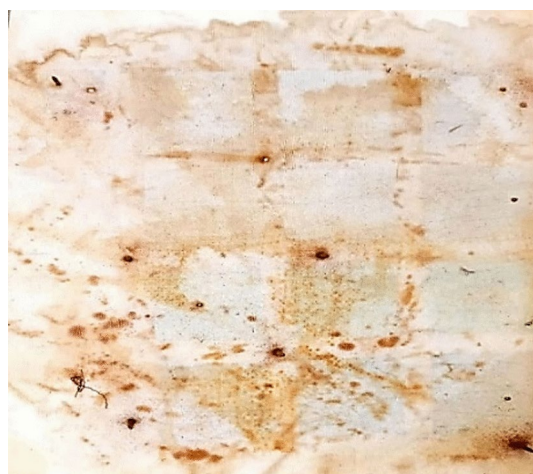
Fig. 4. Effect of rust on the back surface of the color samples.
