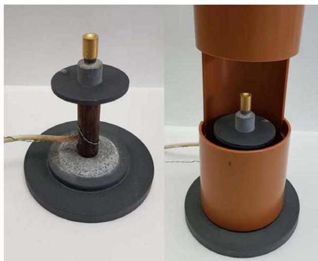
Bullet hot finger assembly with (right) and without (left) extractor hood. The concave surface of the bullet acts as a reaction vessel for the dissolution.
