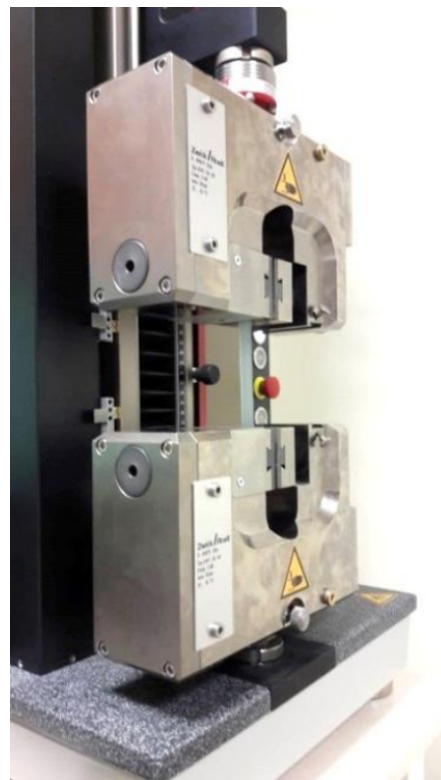
Figure 1. Zwick Z5.0 TN ZwickLine testing machine.
