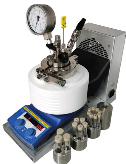
Figure S11. The Wattcas autoclave (WP-MSAR-250A) for solvothermal reactions.
