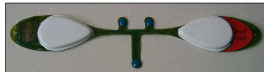
Figure 5: SleepStrip®, airflow is measured with a thermistor
