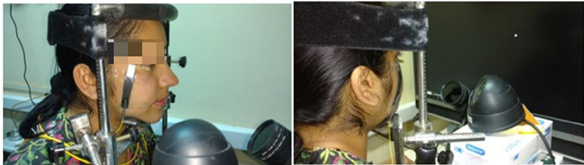
Fig. 5. Experimental Setup with FBGET mounted on the subject and ISCAN placed on a nearby reference plane.
