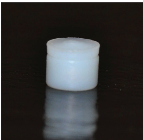
Figure 1: Indigenously fabricated dental magnet
