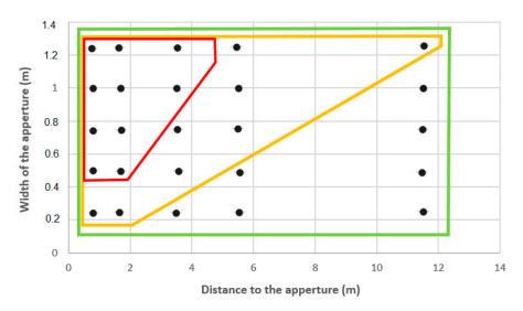
**Figure 5.** Detection performance for apertures, with black points representing points of measurement from different distances. The red parallelepiped contains points indicating apertures detected at 0.8 rad/s; those inside the yellow parallelepiped indicate apertures detected at 0.4 rad/s and the green parallelepiped indicates full aperture detection at 0.2 rad/s.
