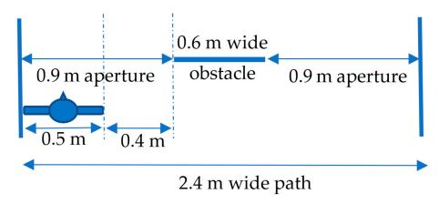
**Figure 6.** Schematic top view of the experimental setup illustrating the parameters used for computing the probability of passing the apertures without collisions by chance.
