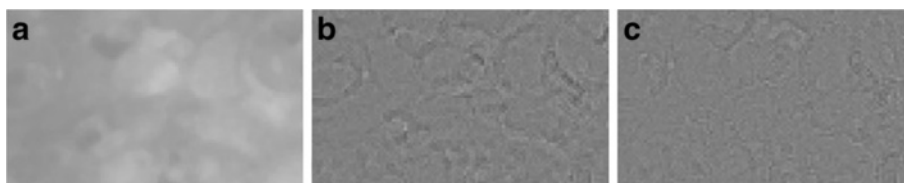
Figure 2 Registration example using wavelet filtering. a ) Differences of misaligned frames at two different wavelengths. b ) Differences of the first wavelet layer, same images (Std dev: 0.025). c ) Differences of the first wavelet layer, after registration (Std dev: 0.021).
