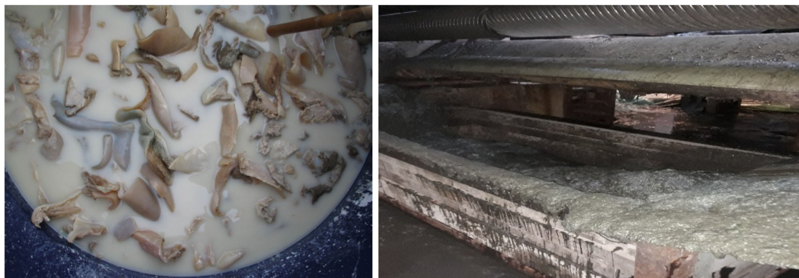
Figure 1. Limed hide waste (gelatin and lime fleshing) at SC PIELOREX Jilava, Romania.
