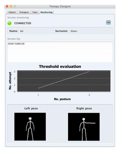
**Figure 6.** NAOTherapist monitoring interface. Real-time information is offered to the therapist, including the step that is currently being performed during the therapy session, a plot showing the number of attempts that the patient needed to complete each posture (information internally used by the architecture to adjust the evaluation threshold), and finally the last position asked of the patient.
