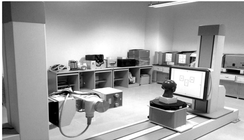
Figure 5. In-house bench-top CBCT system for raw projection acquisition.
