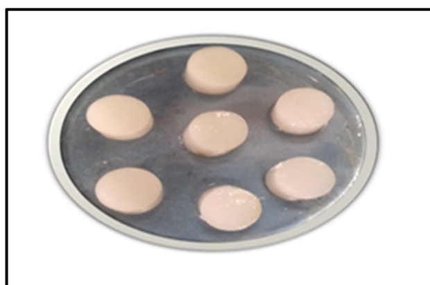
Figure 2. Pluronic acid/agarose-co-poly (methacrylic acid) hydrogels.
