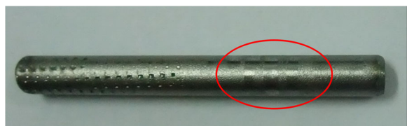
Fig. 5 The failure region of RF-F-10 rod was at the groove of screws but not at the junction of rod inside MTS mechanical testing machine regarding the anti-rotational torque
