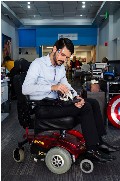
Fig. 1 An overview of the EMG control of motorized wheelchair devices. Pictured is a user utilizing electromyography to control the movement of the joystick via the attachment to the wheelchair device
