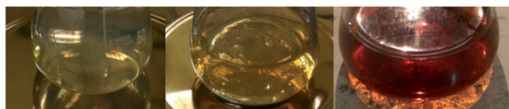
Fig. 4 Successive colour changes with time during the synthesis of silver nanoplates using leaves extract of Eichhornia crassipes .
