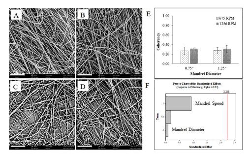
**Fig 2. PNIPAM nanofibers as a function of mandrel diameter and mandrel speed.** (A) 0.75" (19mm) mandrel diameter, 675 RPM. (B) 0.75", 1356 RPM. (C) 1.25" (31.8mm), 675 RPM. (D) 1.25", 1356 RPM. Scale bar (lower left of each image) is 20 μm. Alignment is not affected by mandrel diameter or mandrel speed, as shown in (E) as coherency values and (F) in the analysis of the factorial design.
