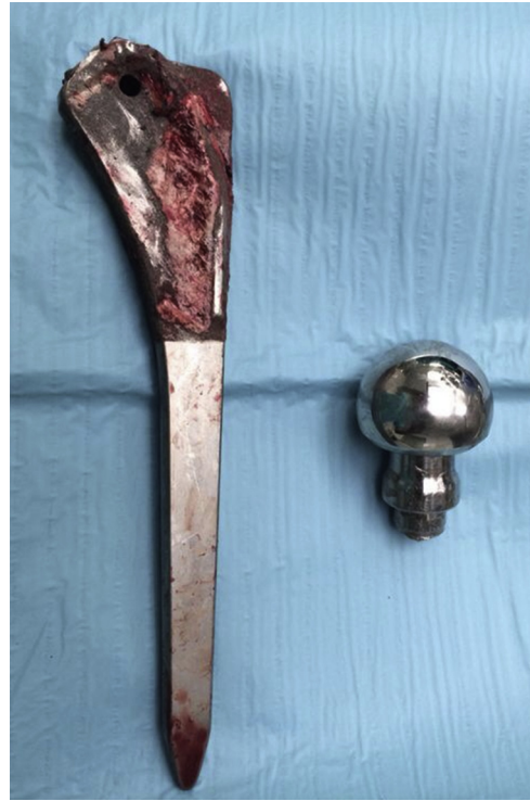
Fig. 5. Macroscopic aspect of the fragments of the Bicontact extracted prosthesis.
