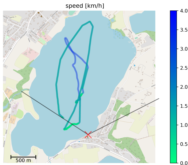
Figure 10. Ground station location (marked by red X), its 3 dB antenna sector boundary and HydroDron movement speed (km/h) during the test deployment.
