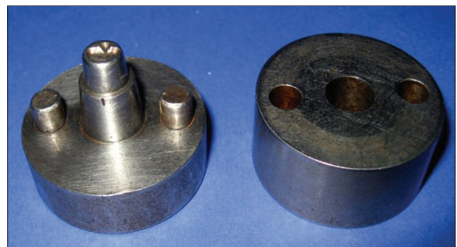
Figure 1: Stainless steel master die and counter
