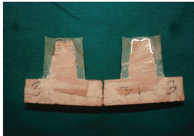
Figure 6: Sectioned coping-die assembly prepared to observe axial wall adaptation
