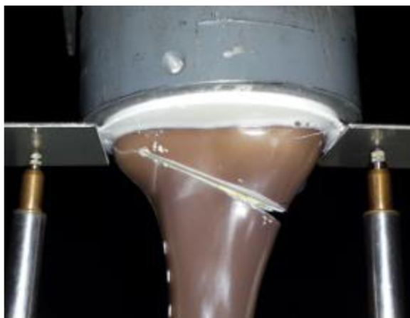
Fig. 6 Cracking of the contralateral cortex during the cyclical testing: Unlike the case of Activmotion 4 showed on the picture, the cracking was generally not observable
