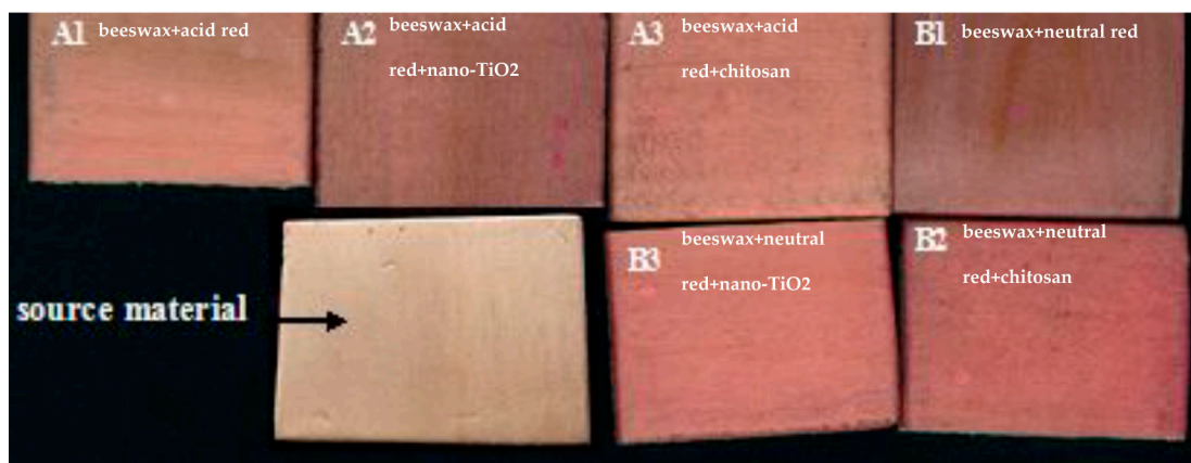
Figure 5. The color change of the modified wax specimen and material surface after 60 h UV-irradiation.
