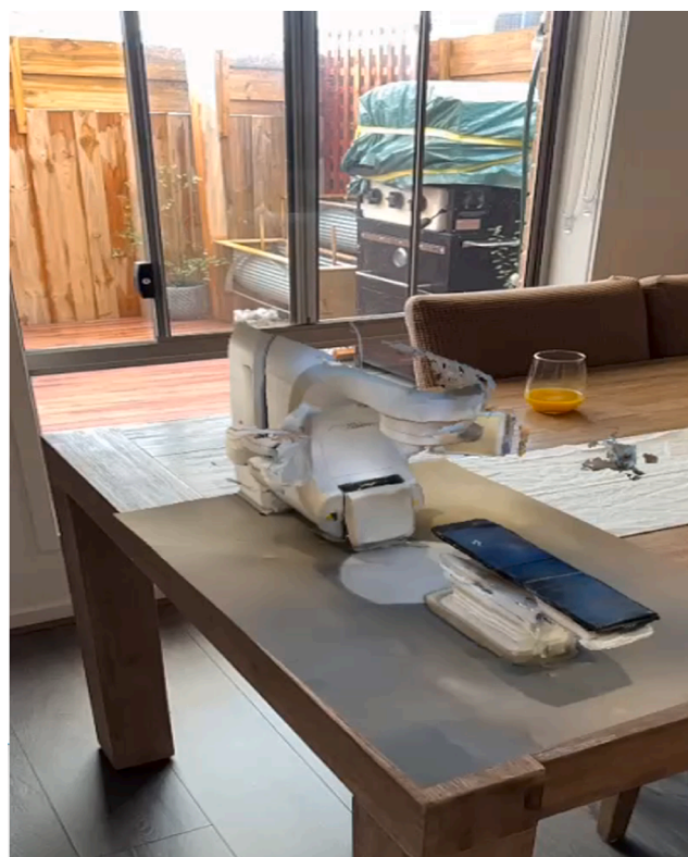
Fig. 4. AR representation of linear accelerator overlaid on a kitchen table.
