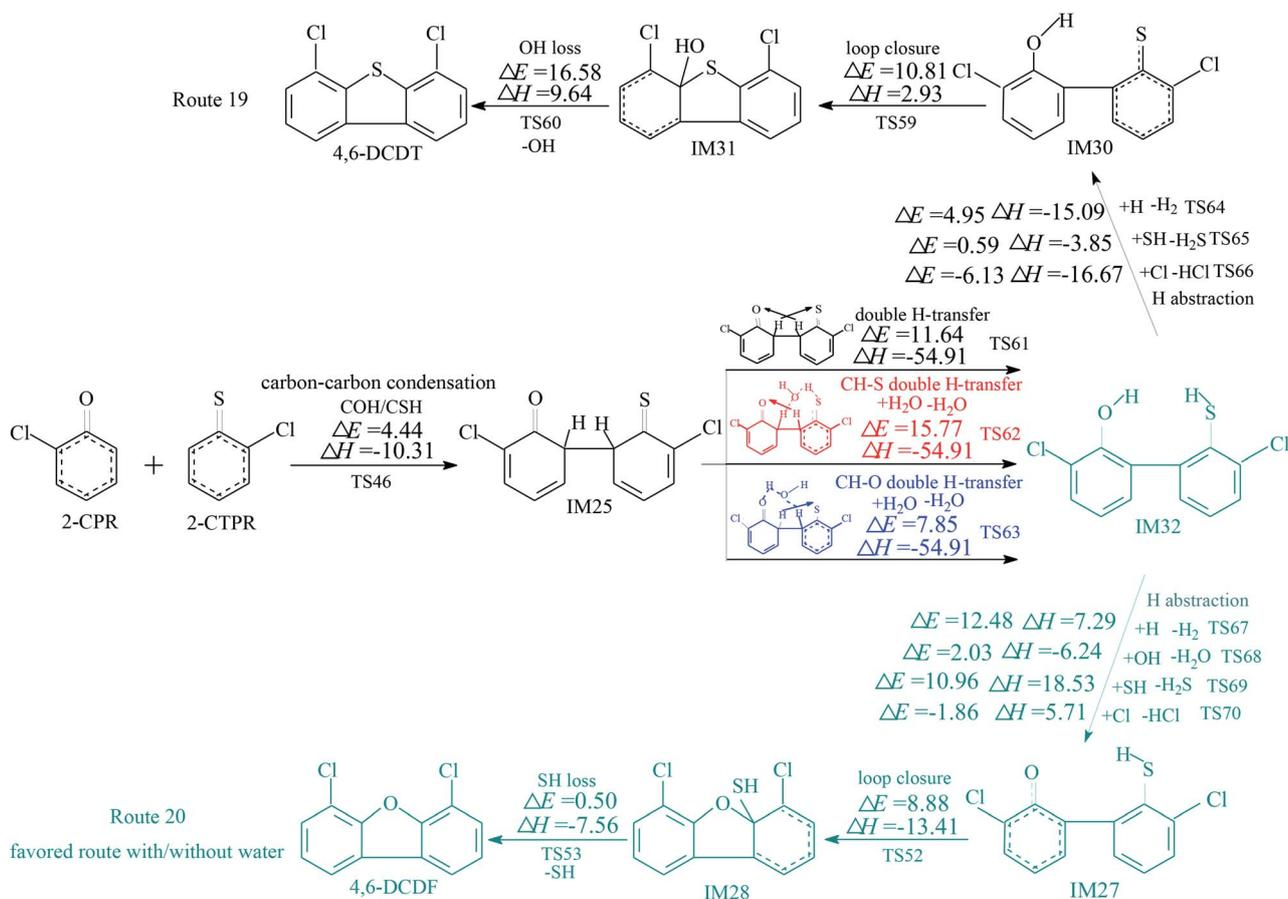
Fig. 4 Formation routes of PCDF/DTs including potential barrier ( $\Delta E$  (in kcal mol<sup>-1</sup>) and reaction heat ( $\Delta H$  (in kcal mol<sup>-1</sup>) values via the carbon-carbon condensation (COH/CSH) of 2-CPR and 2-CTPR with double H transfer steps.  $\Delta H$  is calculated at 0 K. The green route represents the favored route both with and without the introduction of water molecules.
