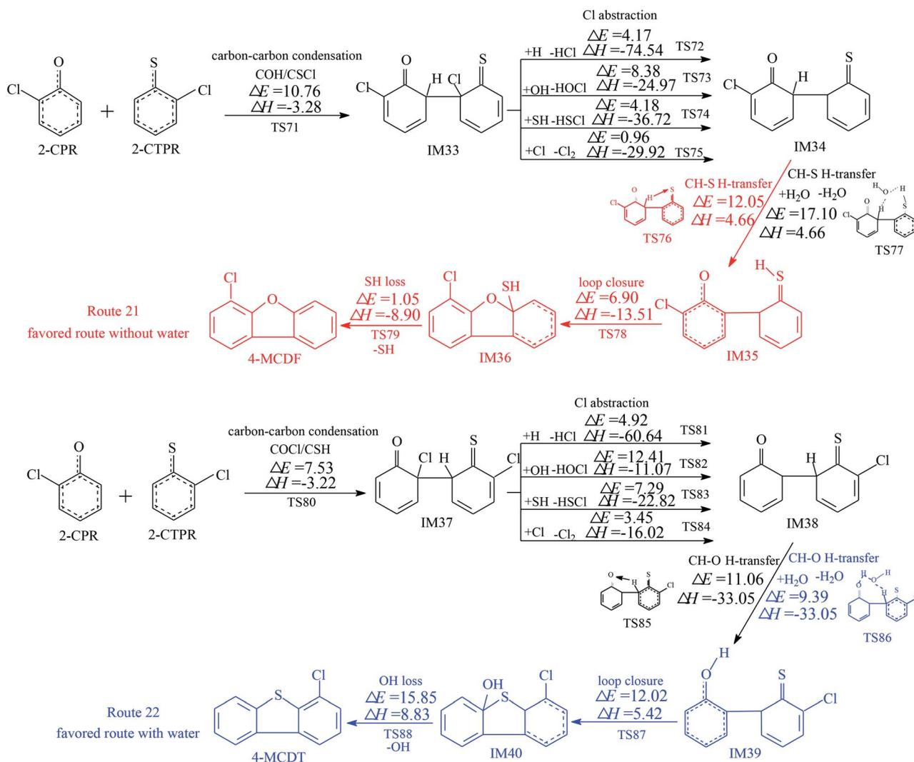
Fig. 5 Formation routes of PCDF/DTs including potential barrier ( $\Delta E$  (in kcal mol<sup>-1</sup>)) and reaction heat ( $\Delta H$  (in kcal mol<sup>-1</sup>)) values via the carbon-carbon condensation (COCl/CSH and COH/CSCl) of 2-CPR and 2-CTPR.  $\Delta H$  is calculated at 0 K. The red route represents the favored route without the introduction of water molecules, and the blue route shows the favored route with the introduction of water molecules.
