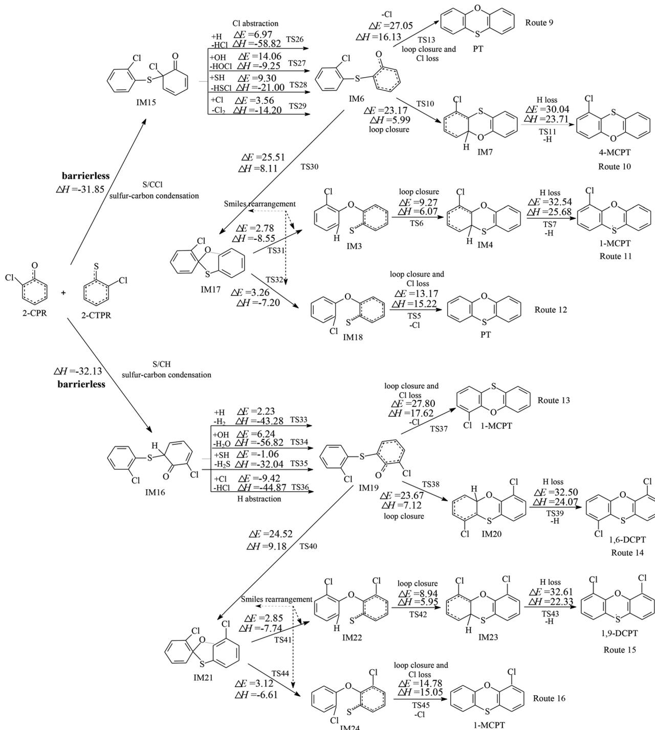
Fig. 2 Formation routes of PCPTs including potential barrier ( $\Delta E$  (in kcal mol<sup>-1</sup>) and reaction heat ( $\Delta H$  (in kcal mol<sup>-1</sup>) values via the sulfur-carbon condensation (S/C/Cl and S/CH) of 2-CPR and 2-CTPR.  $\Delta H$  is calculated at 0 K.
