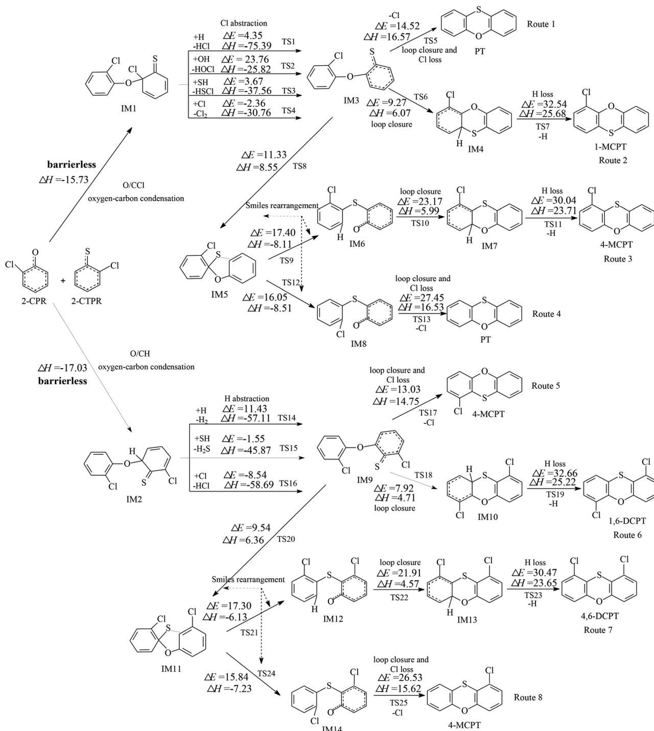
Fig. 1 Formation routes of PCPTs including potential barrier ( $\Delta E$  (in kcal mol<sup>-1</sup>)) and reaction heat ( $\Delta H$  (in kcal mol<sup>-1</sup>)) values via the oxygen-carbon condensation (O/CCl and O/CH) of 2-CPR and 2-CTPR.  $\Delta H$  is calculated at 0 K.
