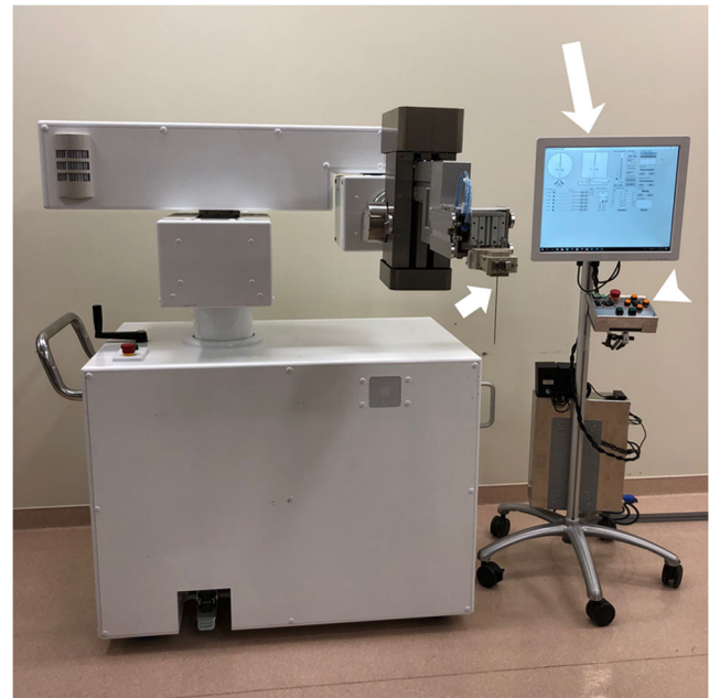
Fig. 1 The robotic system. A robot (left) with 6 degrees of freedom and an interface (right) comprising a touch panel (long arrow) and a controller (arrowhead). The robot may be manipulated by either button operation of the controller or numerical inputs on software displayed on the touch panel. With the former technique, the robot moves while the buttons of the controller are manually pressed, whereas with the latter technique, the robot moves to a certain place semi-automatically after numerical inputs. In the present study, typically, alteration of needle angles for needle targeting and adjustment of needle orientation was performed by the latter, while needle insertion was done by the former. The needle (short arrow) is attached to a plastic needle holder at the end of a robot arm
