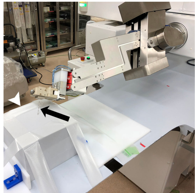
Fig. 2 Robotic out-of-plane needle insertion in the phantom experiment. The needle (arrow) at the predetermined angles in the XY and YZ planes is inserted into a sponge phantom (arrowhead) fixed on the CT table
