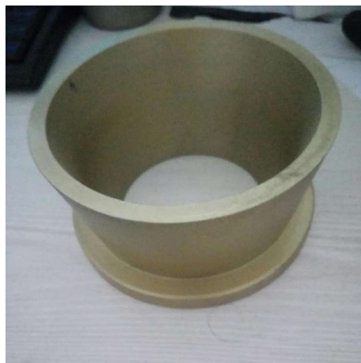
Figure 4. Truncated-cone round die.
