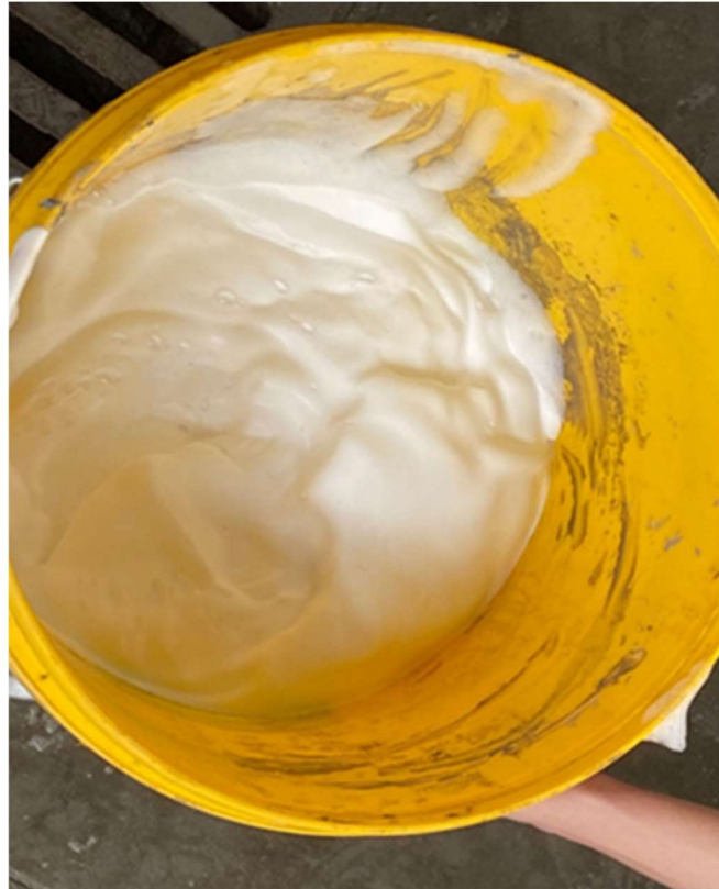
Figure 3. The foam produced by physical foaming with this foaming agent.
