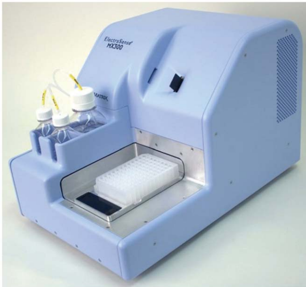
Figure 3. Photograph of the MX300 Automated Microarray Workstation. Reagents are loaded in a 96-well plate, and a programming script is used to control their flow into a single chamber or into four chambers containing an ElectraSense microarray. Current or voltage can be applied to single or groups of electrodes for Ppy deposition, and current can be read from a single electrode or groups of electrodes for ECD.
