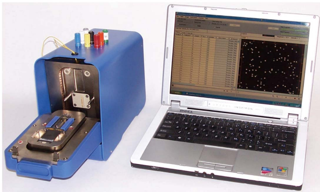
Figure 2. Photograph of the PotentioSense Workstation with computer. This modified ElectraSense reader has externalized leads on the case, which provide connections between electrodes on the array and a potentiostat or other external power source.
