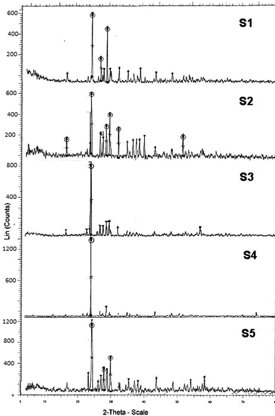
Fig. 4. X-ray diffraction spectra of Gandhaka samples.
