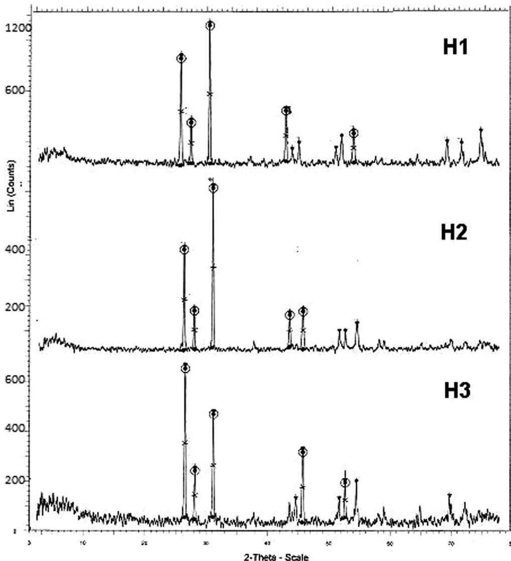
Fig. 6. X-ray diffraction spectra of Hingula samples.
