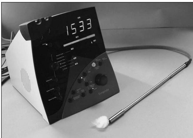
Figure 1. Eurorad's opto-nuclear endoscopic probe and readout module.
