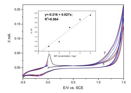
**Figure 3.** Cyclic voltammogram recorded on HKUST-CNF electrode in 0.1 M Na<sub>2</sub>SO<sub>4</sub> supporting electrolyte (curve 1) and in the presence of various IBP concentrations: curves 2–7: 1–6 mg·L<sup>-1</sup> IBP; potential scan rate: 0.05 V·s<sup>-1</sup>; potential range: -0.5 to +1.5 V/SCE. Inset: Calibration plots of the currents recorded at E = +1.25 V vs. SCE versus IBP concentrations.
