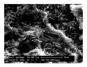
Figure 1. SEM image of the HKUST-CNF composite electrode.
