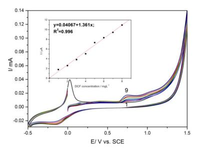
**Figure 2.** Cyclic voltammogram recorded on HKUST-CNF electrode in 0.1 M Na<sub>2</sub>SO<sub>4</sub> supporting electrolyte (curve 1) and in the presence of various DCF concentrations: curves 2–9: 1–8 mg·L<sup>-1</sup> DCF; potential scan rate:  $0.05~\rm V\cdot s^{-1}$ ; potential range:  $-0.5~\rm to$  +1.5 V/SCE. Inset: Calibration plots of the currents recorded at E = +0.75 V vs. SCE vs. DCF concentrations.
