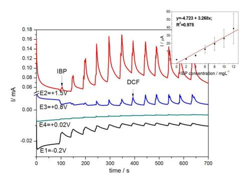
**Figure 8.** Multiple-pulsed amperograms recorded at HKUST-CNF electrode in 0.1 M Na<sub>2</sub>SO<sub>4</sub> supporting electrolyte, consecutively and continuously adding each of 2 mg·L<sup>-1</sup> IBP and respective, DCF, recorded at E1 = -0.2 V/SCE, E2 = +1.5 V/SCE, E3 = +0.8 V/SCE, E4 = +0.02 V/SCE. Inset: Calibration plots of the currents recorded at E = +1.5 V vs. SCE versus IBP concentrations.
