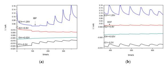
**Figure 5.** Multiple-pulsed amperograms recorded by HKUST-CNF electrode in  $0.1 \text{ M} \text{ Na}_2\text{SO}_4$  supporting electrolyte and adding consecutively and continuously: (a)  $2 \text{ mg} \cdot \text{L}^{-1}$  IBP, recorded at E1 = -0.2 V/SCE, E2 = +0.8 V/SCE, E3 = +1.25 V/SCE, E4 = +0.02 V/SCE; (b)  $2 \text{ mg} \cdot \text{L}^{-1}$  DCF, recorded at E1 = -0.2 V/SCE, E2 = +0.8 V/SCE, E3 = +1.25 V/SCE, E4 = +0.02 V/SCE.
