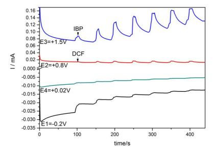
Figure 7. Multiple-pulsed amperograms recorded with a HKUST-CNF electrode in 0.1 M Na<sub>2</sub>SO<sub>4</sub> supporting electrolyte and continuously adding a mixture of 2 mg·L<sup>-1</sup> DCF and 2 mg·L<sup>-1</sup> IBP, recorded at E1 = -0.2 V/SCE (time duration of 0.5 s), E2 = +0.8 V/SCE (time duration of 0.5 s), E3 = +1.25 V/SCE (time duration of 0.1 s), E4 = +0.02 V/SCE (time duration of 0.5 s).
