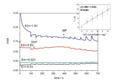
**Figure 9.** Multiple-pulsed amperograms recorded at HKUST-CNF electrode in 0.1 M Na<sub>2</sub>SO<sub>4</sub> supporting electrolyte and consecutively and continuously adding each of 2 mg·L<sup>-1</sup> DCF and respective, IBP, recorded at E1 = -0.2 V/SCE, E2 = +0.8 V/SCE, E3 = +1.5 V/SCE, E4 = +0.02 V/SCE. Inset: Calibration plots of the currents recorded at E = +0.8 V vs. SCE versus DCF concentrations.
