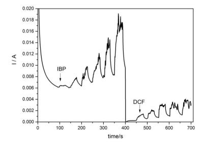
**Figure 6.** Amperometric response at the HKUST-CNF electrode for the six successive and continuous additions of 2 mg·L $^{-1}$  IBP recorded at +1.25 V vs. SCE for 400 s running time followed by the five successive and continuous additions of 2 mg·L $^{-1}$  DCF at applied potential of +0.8 V vs. SCE for the next running time of 400 s.
