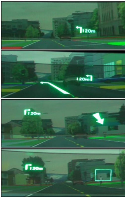
Fig. 10. Different types visualizations for an in-vehicle AR-HUD as investigated by Bolton et al. [45]. (Republished with permission of ACM (Association for Computing Machinery), from An investigation of augmented reality presentations of landmark-based navigation using a head-up display , Large, David R; Burnett, Gary; Bolton, Adam, 2015; permission conveyed through Copyright Clearance Center, Inc.)
