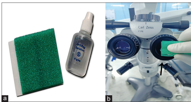
Figure 2: (a) Image depicting medical-grade anti-fog solution with an anti-scratch sponge for cleaning the microscope eyepieces. (b) Image depicting microscope eyepiece being cleaned with an anti-scratch sponge after anti-fog solution application (black arrowhead)
