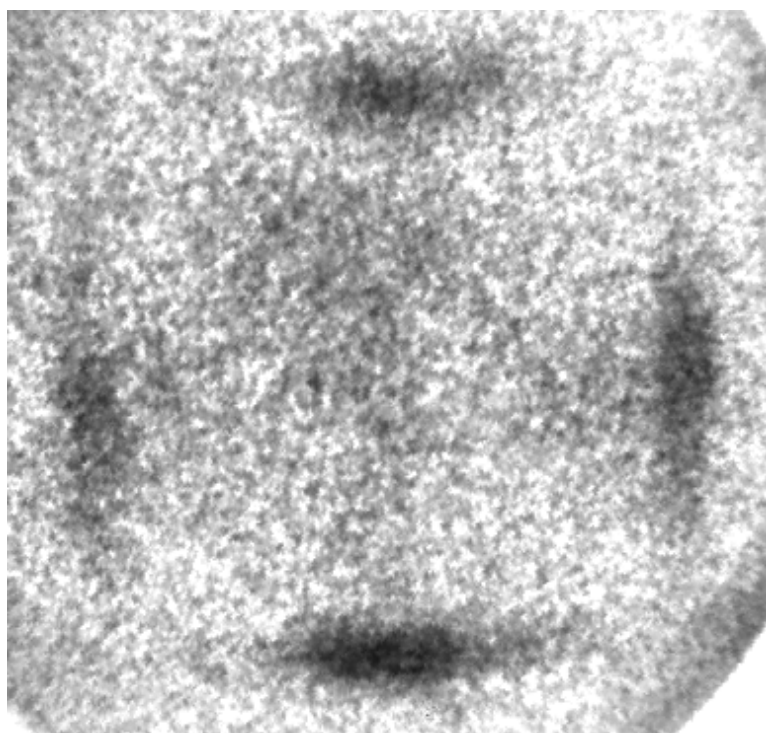
Figure 6. Equi-energy cut at Fermi level of single a-a twin domain. The non-vanishing intensity around \bar{\Gamma} point is apparent. The noisy nature of the image originates from an extremely small area available for analysis.
