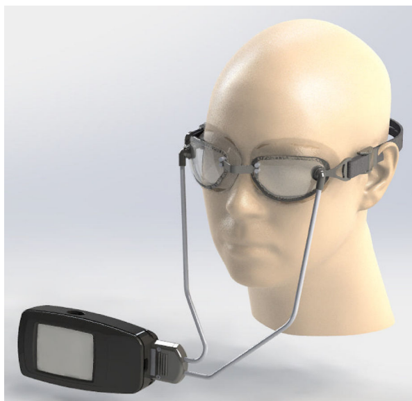
Fig. 1 Standard iteration of the multi-pressure dial (MPD), which consists of a pair of pressure-sensing goggles connected to a pressure-modulating pump
