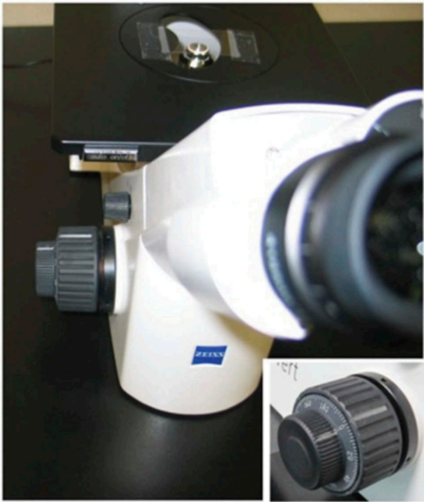
Figure 1. Setup for the matrix height measurement. A line was marked on both the fine and coarse focus knobs to facilitate unit measurements. Note the clockwise sequence of numbers on the fine focus knob (inset) requiring downward focusing movement to measure increasing distances.
