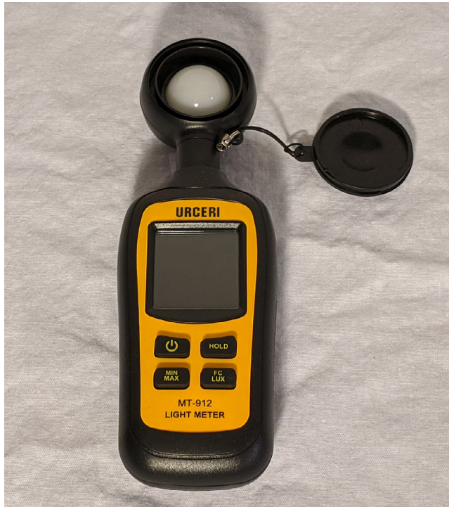
Fig. 6. Urceri MT-912 light meter used for luminance testing.
