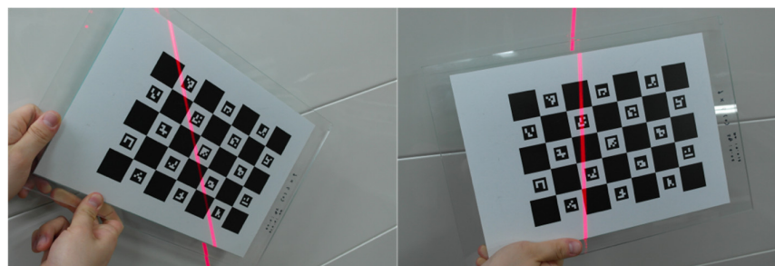
Figure 6. Calibration of laser plane with respect to camera coordinate.
