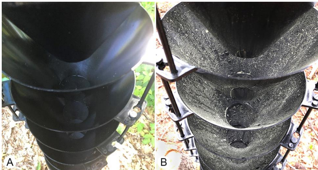
Figure 1. Example of multiple-funnel trap treatments from Experiment 1 in a mixed conifer stand in southeastern New Hampshire. (A) Clean trap without surfactant switched out biweekly with a clean trap; (B) Control trap without surfactant after six weeks in the field (not shown: two additional treatments of surfactant-treated clean trap and surfactant-treated control trap).
