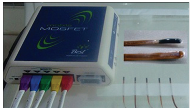
Figure 1: Photograph of Mobile MOSFET dose verification system with brass build-up cap
