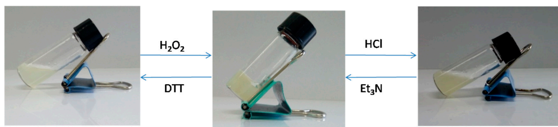
Figure 6. Sol-gel transitions of PEG-DTP/ADA hydrogels in response to pH or redox triggers.
