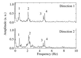
Table 1 presents the peak natural frequencies from Figure 8, obtained experimentally with the optical accelerometer in the tower, for both measured directions.
