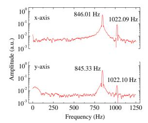
**Figure 3.** Frequency response of the accelerometer for both sensitive directions.
