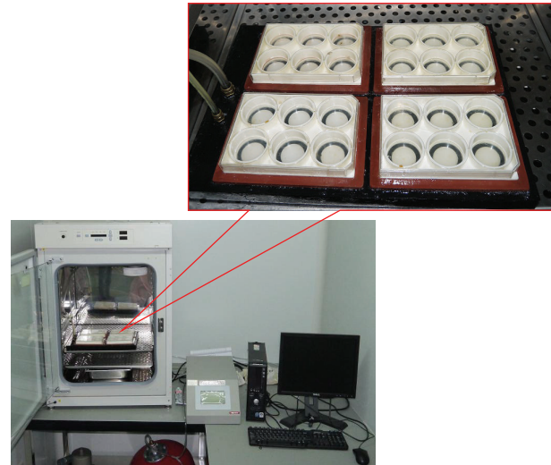
FIGURE 1: The Flexcell-5000 cell mechanical appliance was used. Cells were cultured in 6-well culture plates containing an elastic silicone membrane and fixed to the appliance module. A rubber gasket and silicone gel were applied to seal the gap between the modules and plates. A vacuum pump was connected to the module to generate negative pressure and induce periodical concave movement in the elastic membrane at the culture plate bottom. Thus, a force was applied along the surface of the radial tangent membrane to stimulate the cells attached to the membrane by the stretching stress. Tension was calculated by converting the stretching magnitude of the silicone membrane from its deformation rate (%).
