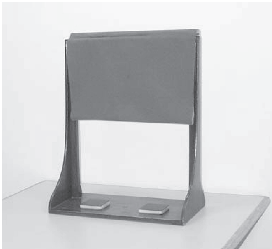
Figure 1 A modified Wisconsin General Test Apparatus (WGTA). The WGTA consisted of a wooden frame approximately 54 cm wide and 65 cm high. An opaque curtain was anchored to the top of the frame in such a way that it could be raised by the experimenter to reveal a stimulus board (53 x 28 cm) containing two circular reinforcement wells 8 cm in diameter and 1 cm deep. The reinforcement wells were covered with felt cloth to eliminate auditory cues associated with coin placement and the preparation of each trial. The reinforcement wells were 24 cm apart from center to center, and for DA tasks, the wells were covered by identical black square stimulus plaques (7.6 x 7.6 x 0.5 cm). For OA tasks, a three-dimensional stimulus object (eg, a small toy) was mounted on each plaque; each of the objects had different shapes and colors. When the curtain was in the lowered position, the participant could see neither the stimuli nor the investigator. When the curtain was raised for each trial, the participant could see the stimuli and the hands of the investigator, but not the investigator's face.
